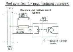
waveform. This can cause the EIA485 devices to produce errors. The safest use of a DOL device is as the only receiver, or a small number of receivers, at the end of the line.
