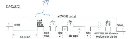
The other 255 different possible start-codes are not defined by DMX512, although some have been reserved. Some manufacturers use non-zero start-codes to send additional information unique to their products. Future enhancements to the DMX512 specification will use alternative start-codes, for instance for error checking and 'talkback' or to send data other than levels. Compatibility is ensured, however, as start-code zero will always indicate 8 bit level information.
