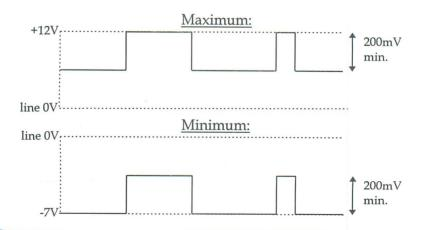
Important: If common-mode voltage exceeds these limits, damage may be caused to both the transmitter and receiver circuits.
