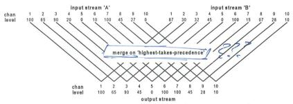
A typical use for such a system is when moving lights are controlled from one type of desk and conventional dimmers from another. Merging computers simply merge the channels one-by-one from the two input streams, the higher value present on either stream being the one that prevails ('highest-takes-precedence').
