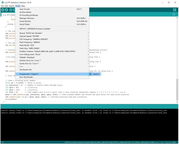
It's important to note that after the code is uploaded, the device will start to run it. So, if we want to upload a new program, wee need to reset the power of the device, in order to guarantee that it enters flashing mode again.
