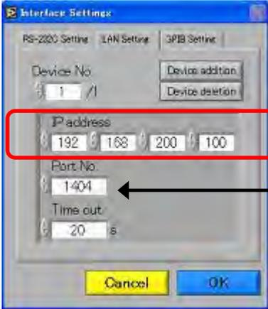
← Check IP address at COMM SETUP window of RA2300A.
