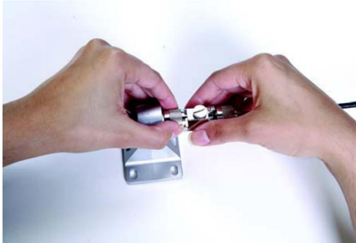
**STEP 3** Attach the taped end of the antenna cable to the Wireless-G Exterior Access Point.
