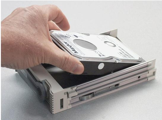
2. Carefully place a Serial ATA disk drive into the drive carrier and slide it all the way to the back.
