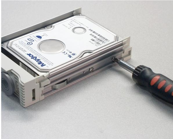
3. Install and tighten the four mounting screws to secure the disk drive in the drive carrier.
