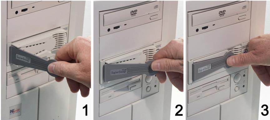
5. Carefully slide the drive carrier into the housing assembly with the handle turned out all the way.
