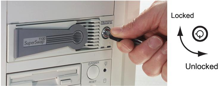
7. Insert the key and turn it 90 degrees clockwise to lock the drive carrier in the enclosure.
