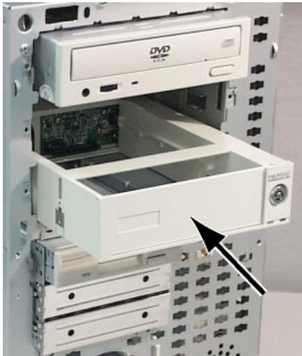
**Figure 1.** Slide the SuperSwap enclosure into a drive bay.
