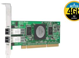
QLA2462 Host Bus Adapter. The QLA2462 is the industry's first, true enterprise class, 4-Gbps to PCI-X 2.0 HBA. The QLA2462 not only delivers unprecedented levels of performance and availability, but also intelligent networking features specific to enterprise class data centers.
